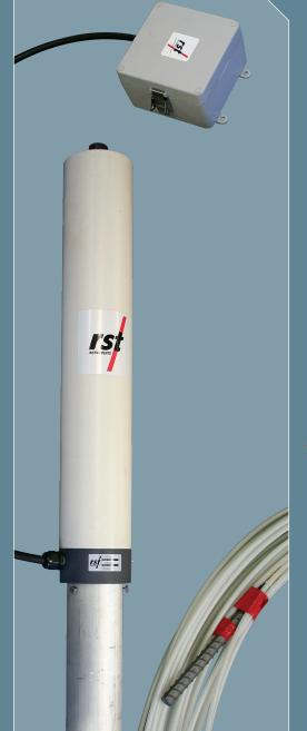
A low cost, convenient instrument for the monitoring of ground displacements. Designed to withstand severe field conditions and accommodate transverse shear. The unit is supplied completely assembled and sealed for grouting into the borehole. Rod displacement readings may be taken manually using a dial gauge or monitored continuously with a remote readout head.
