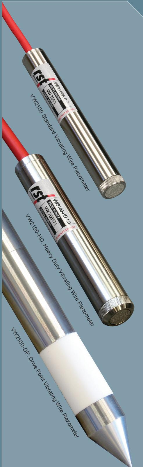
The RST Vibrating Wire Piezometer provides excellent long-term accuracy, stability of readings and reliability under demanding geotechnical conditions. Vibrating Wire Piezometers are the electrical piezometers of choice as the frequency output of VW devices is immune to external electrical noise, and able to tolerate wet wiring common in geotechnical applications.
