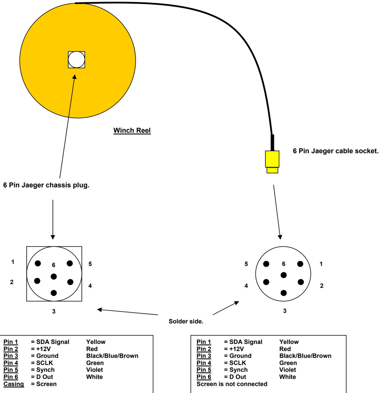
**Fig 7. General Connection Arrangement**
