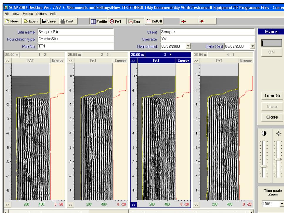
You can choose to display the first arrival time trace (FAT) and the signal energy (ENG) by clicking the buttons on the top of the page. The contrast and brightness of signals can be altered using the contrast sliders at the bottom right of the display.
