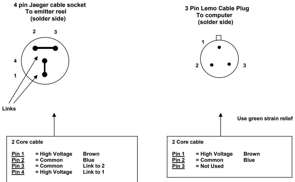
**Fig 3. Cable From Site Computer To Receiver Reel.**
