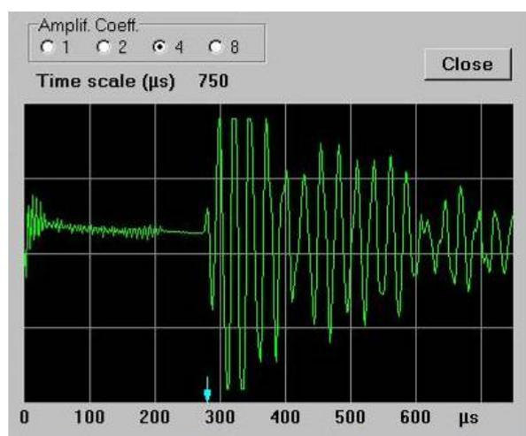
This shows the signal at the current probe position. The amplitude can be altered by selecting a suitable coefficient. Aim to just fill the screen. The time base can also be altered in this mode. You will need to press the stop button on the screen first.. Aim for the first arrival to be about two thirds of the full scale . Click on close and the box will disappear. If there is no signal, the probes may not be level, or one tube is blocked. Press top winch button to stop.
