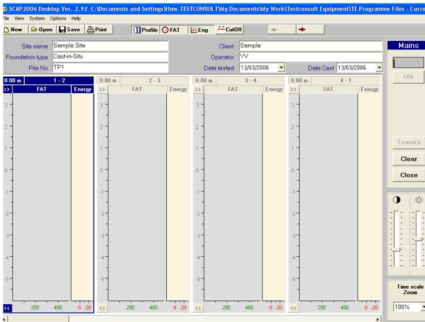
Once all of the cables are connected, click on the Mains - On button to activate the acquisition board and the winch. The box below mains will go green and a line should move from side to side if the winch is communicating with the computer.
