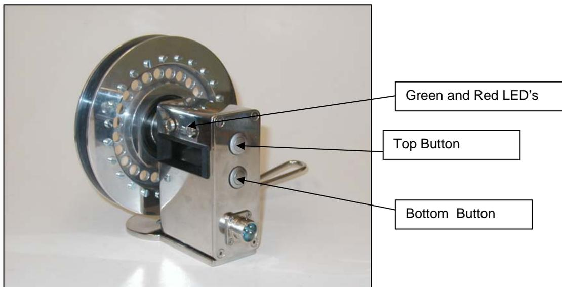
There are two buttons on the side of the winch which allow the operator to control the testing and data storage operation without having to keep returning to the testing vehicle and the computer. There are three different modes as follows:
